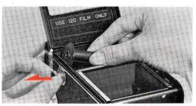
You will probably find an empty takeup spool in the lower chamber. Pull out the Spool Supporter (Lower) and remove the spool, and place it in the upper chamber by pulling out the spool Supporter (Upper) and slipping the spool in. Then release the supporter so that it snaps back in and holds the spool securely.
