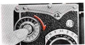
After you have taken the first exposure, depress the Film Transport Release Button in the center of the Film Winding Knob, then turn the knob until it stops. You will note that the figure "2" appears in the Exposure Counter. You are, of course, now ready for exposure two. Continue this action for each of the 12 exposures.
