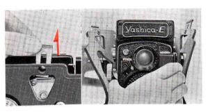
To load the camera you will first have to remove it from the leather case. To do so, pull up the two metal lock slides at the top of the case so they disengage from the Strap Holders. Then spread the sides of the case apart and lift the camera out.
