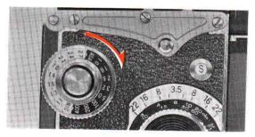
Note that the Exposure Counter is automattically set to "S" (start) when the back cover is closed and locked.
